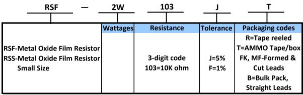
Note: 52, 63 and 73 MM taping are available for different Wattages
